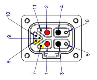
Insert the temporary wire to bridge pins 7 & 8 like shown below.
