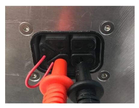
MULTIMETER PROBES IN PINS 1 & 3
