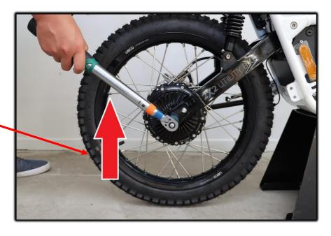
Apply Loctite and torque to 90Nm
