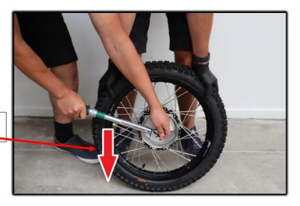
Torque is applied in a downwards direction
