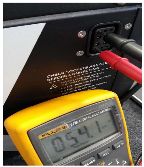
**NOTE:** When the battery is charged it should be between 57.6-58.8 volts and a flat battery will be 38.8 - 43 volts. To afford unwanted repair times ensure your battery is charged when working on your UBCO 2x2.
