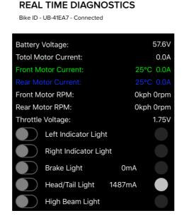
The top section of advanced diagnostics allows real-time visualisation of selected bike parameters, and the ability to control bike parameters for testing.
