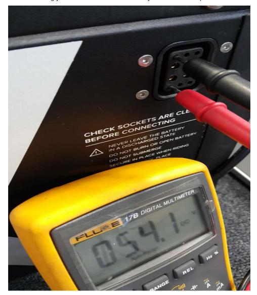
Testing battery voltage for any battery. Charged it should be between 52-58 volts
