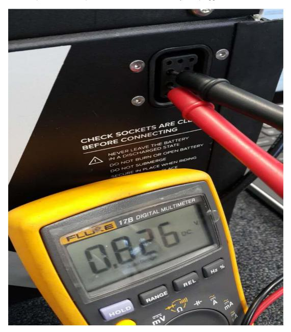
If BMS has failed and latched on this will read the same as pic 1.
