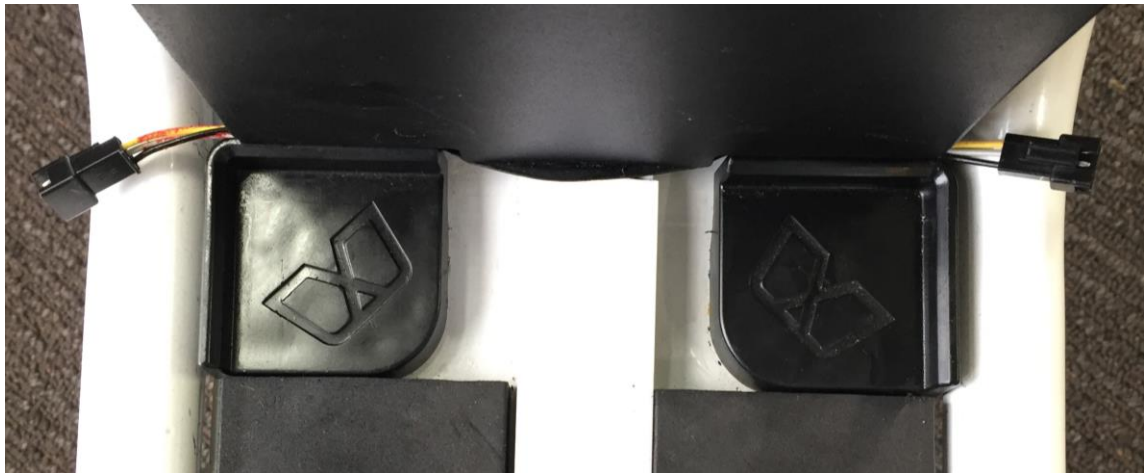
Figure 3 Slide the plugs to the side of the bike as above.
