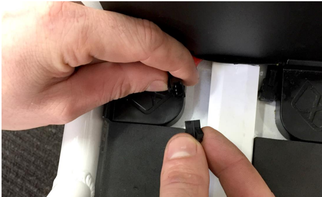
Figure 11 Replace end plugs into cable connector.
