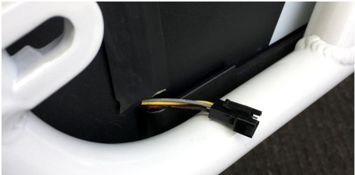
Figure 4 Replace the battery ensuring the cables are accessible as illustrated.
