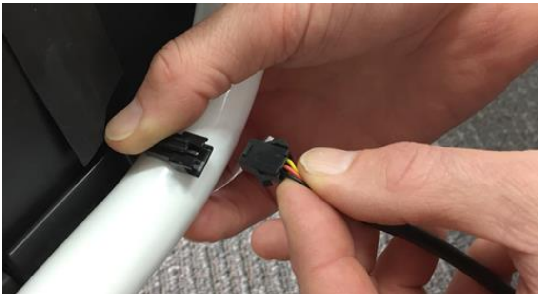
Figure 5 Plug USB cable into the controller cable.
