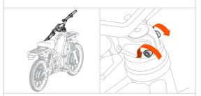
Once the handlebars are straight, re-tighten the stem bolts, alternating as you go to prevent damage to the clamp. Align the marking on the bolt head to achieve the correct tightness. Torque to 15Nm, if available.
