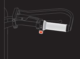
Press the red button to enable Drive. The headlight will turn on. Twist the throttle towards you to go.
